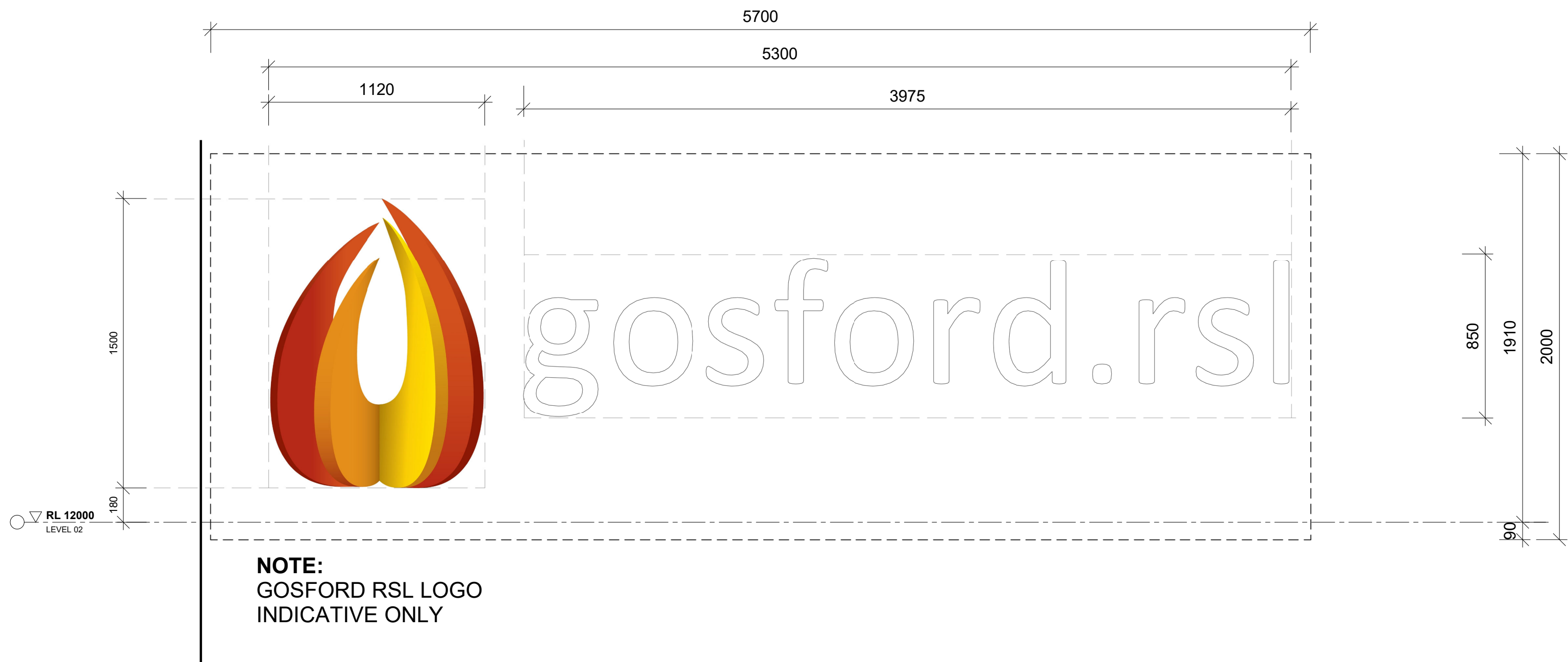
2 SIGNAGE - DETAILED WEST ELEVATION SCALE 1 : 20
